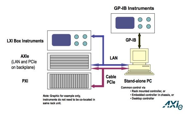
AXIe systems rarely operate alone. Often they are complemented by traditional instrumentation or modular instruments such as PXI in a rack. The diagram above shows how AXIe communication is integrated with LXI, PXI, and GP-IB instruments. Though the figure shows an external PC, the controller may alternatively be embedded within the AXIe or PXI chassis.
