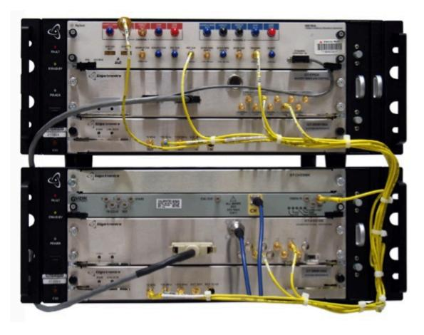
The AXIe system shown above shows two specialized AXIe chassis from Giga-tronics housing Giga-tronics, Guzik, and Keysight modules to build a closed loop EW tester. Each chassis may be used standalone to perform transmitter or receiver testing.
