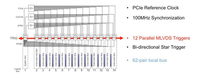
It should be noted that the "system slot" mentioned above may be an actual slot, or embedded in the chassis. Typically, 2 and 5 slot chassis have the system functionality included within the chassis, while 14 slot configurations have a specified AXIe slot that a system module plugs into.
